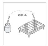
Mix protease with lysis buffer and lysing agent 2 and dispense 200  $\mu L$  of solution into cluster tubes.
