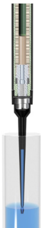
Figure 3–1: Air displacement pipetting principle
